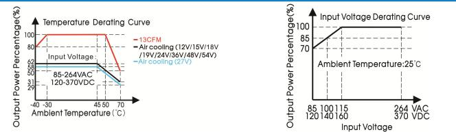
Note: With an AC input voltage between 85-115VAC and a DC input between 120-160VDC the output power must be derated as per the temperature derating curves.
